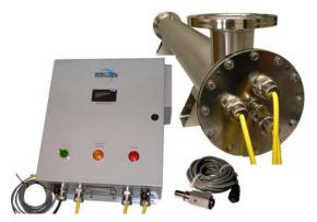
The electropolished, 316L stainless steel or CPVC UV Reactor houses more lamps per volume of flow than MP. This provides a more uniform UV intensity field and inherent degree of redundancy. Consider the situation where a single lamp fails in a 2-lamp MP system versus an 8-lamp amalgam lamp system.
